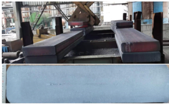
图1 Cr12MoV 钢 150 mm×630 mm 连铸坯实物和低倍 Fig. 1 150 mm×630 mm Continuous casting billet and macro-structure of Cr12MoV steel
